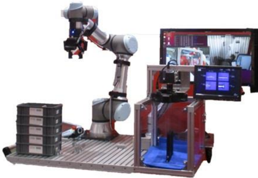
A collaborative robot (Assembly by ASCe of the Punch Group)
